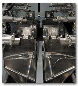
Surge hoppers can be built to different hold capacities (Typically 5, 10, and 15 cubic foot hold capacity) and are available in carbon steel or 304 stainless steel. Each hopper includes a hinged cover lid with handle and gas springs to assist in opening and closing. Most of our systems employ multiple hoppers in a range of sizes.
