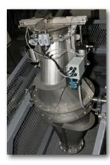
Tumblers are provided to mix all of the preweighed ingredients and utilize variable speed control to control the speed and duration of the mixing. A specially-designed discharge gate, pneumatically actuated with locks and sensors for monitoring, is used to load and unload the tumbler.
